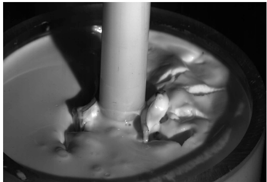
FIG. 2. An example of cracking in a dense suspension (the right portion of the container). The center rod and extrusion apply a shear stress that jams the suspension and causes it to exhibit the solid-like behavior of cracking.
